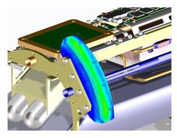
Simulate and analyze designs under stress and thermal conditions with PTC Creo Elements/Direct FEA.
