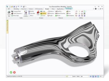
Leverage Creo Elements/Direct Surfacing to dynamically analyze surfaces and visualize curvature.
